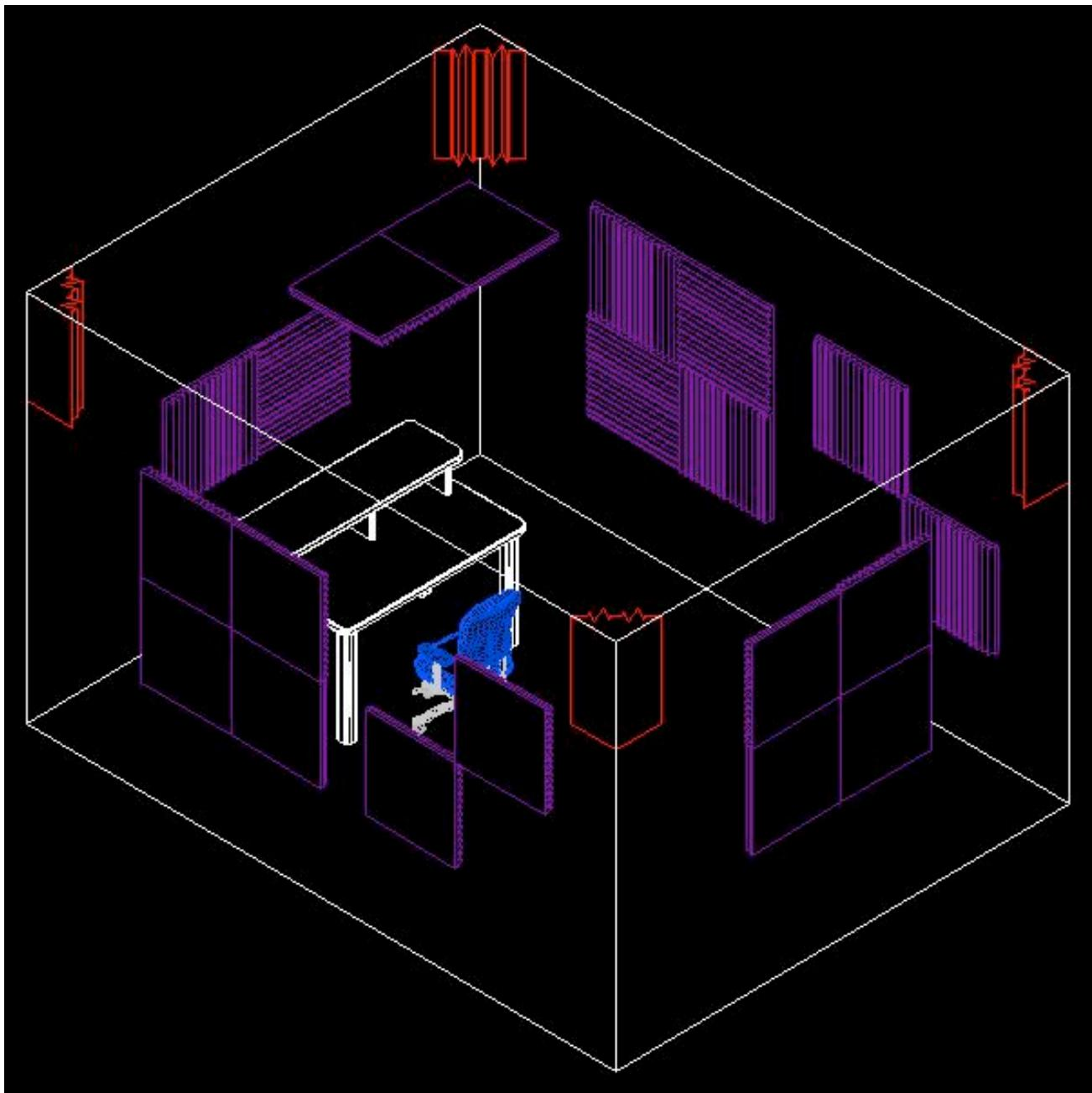
The pattern shown in this rendering is only one example of the way that the panels and bass traps of your Saturn 3 kit can be oriented in the room. If you desire a different aesthetic pattern, you can rotate the panels however you like as long as the guidelines listed above are followed as this will not detract from the performance of the acoustic treatment.
