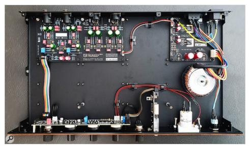
On the inside, you'll find separate PCBs for the power supply (top right), the main audio processing circuitry (top left) and the main front-panel controls (bottom).
